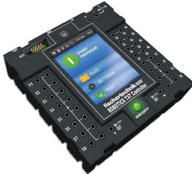
1. The most important requirement of the new fischertechnik TXT controller (part no. 522429 or 153513) is the power supply! Always ensure that you have a charged battery or, preferably, use a mains adapter especially during important operations such as firmware upgrades. A supply voltage of 8~10 Volts is required. Important: ensure that a minimum of 8V is maintained even when outputs are turned on!
