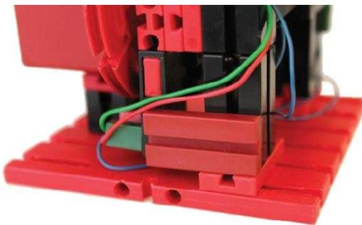
Fig. 11: Securing the end position switch against movement
