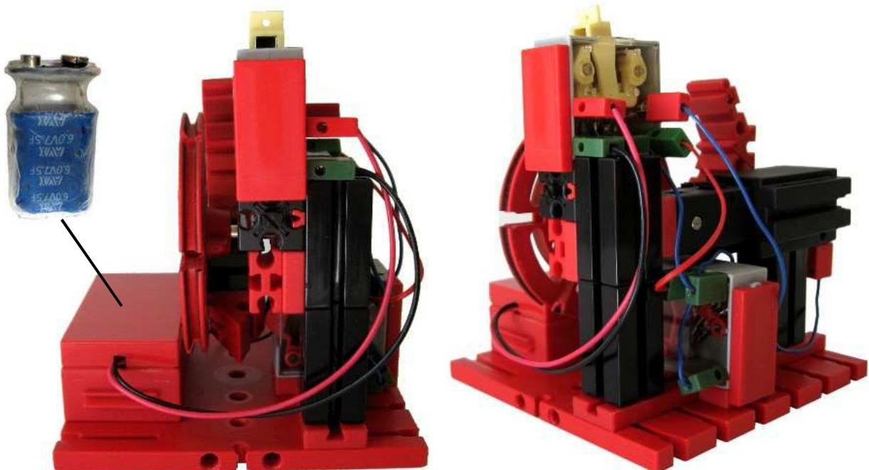
By connecting fischertechnik sockets to pins "1" and "2" of the Polarity Switch, you can recharge the Supercapacitor using a 6V, 1A constant-current limited power supply in less than 30 seconds, without having to remove it from the Useless Machine... your machine is then ready-to-go again in no time... amazing!
