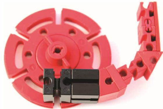
Fig. 3: Turntable with "finger" in rest position.
