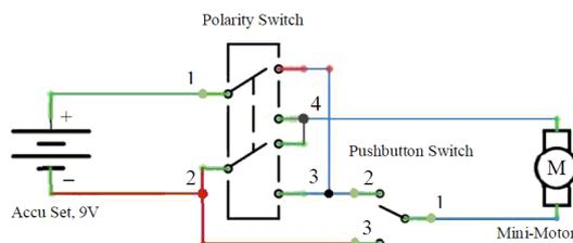
Fig. 5: Circuit diagram of the Useless Machine
