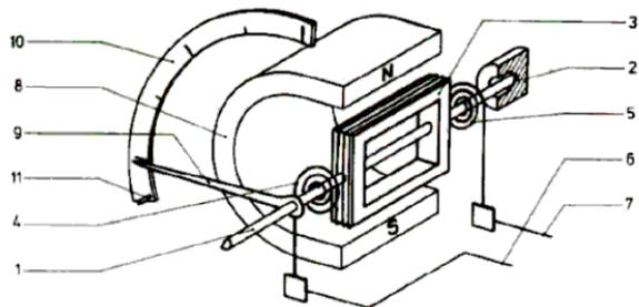
The instrument's measuring unit is mounted on a shaft 1 with "tips" at each end; one tip is inserted into the rear bearing 2 and the other into the front bearing (not shown). The coil 3 is wound with several 1000 turns of the finest enameled copper wire and is electrically connected to two external terminals 6 and 7 via two spiral springs 4 and 5 that are insulated on the shaft. The coil is located between the north and south poles of a permanent magnet 8.
