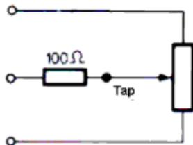
A potentiometer can be used as a voltage divider or as a variable resistor. In the latter case, only 2 terminals are connected.
