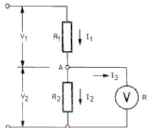
At point "A", the current flowing through the resistor  $R_1$  branches into 2 partial currents. Only if the partial current  $I_3$  flowing through the voltmeter is significantly smaller than the partial current  $I_2$ , the voltage  $V_2$  to be measured changes so insignificantly that the change of this voltage by the connection of the voltmeter is considered negligible.
