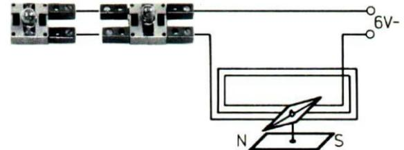
This principle is reversed in the type of electrical measuring device called a "moving-coil meter" which is often used in industry. The coil is mounted in a movable manner and the permanent magnet remains fixed.
