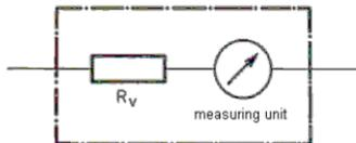
We have called the resistance of the coil pickup of the measuring unit " $R_U$ " and the connected series-resistor as " $R_V$ ". The sum of the two corresponds to the internal resistance " $R_i$ " of the voltmeter or  $R_i = R_U + R_V$ .
