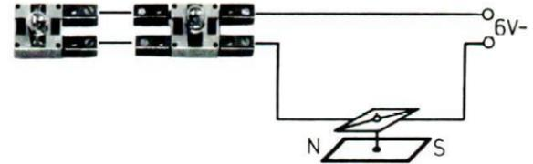
The electrical wire should be passed as near as possible above or below the magnetic needle.
