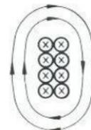
When the wires are wound into a coil, the magnetic fields of the respective opposite wires add to a common magnetic field inside the coil because the opposing wires carry current in the opposite direction. The figure below shows a coil in longitudinal cross section.
