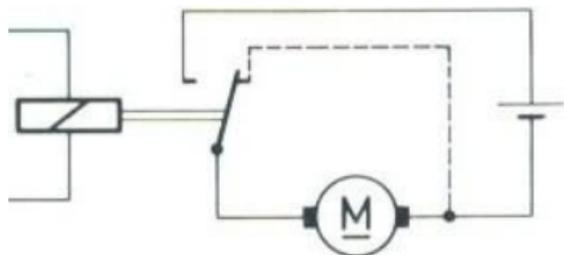
A frequently used circuit in motor control is the polarity reversal.
