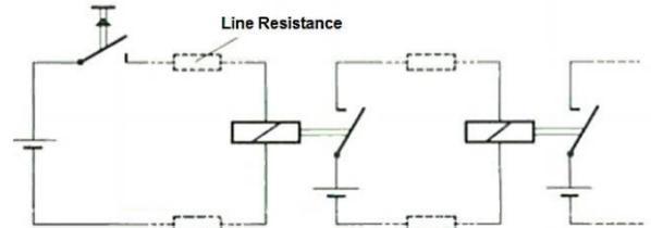
2.) Decoupling (isolation between 2 circuits) The relay can be used to ensure the control circuit and the switching circuit are independent of one another. That is, for example, if a control circuit fed with DC voltage is to switch a load which is supplied with alternating voltage. The same applies if different voltages are applied in the control and switching circuit.
