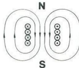
Since iron has a much better conductivity for magnetic field lines than air, the magnetic effect of the magnetic coil is again significantly increased by inserting an iron core.
