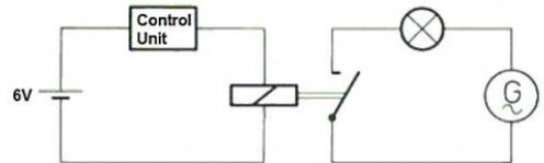
Logic and memory functions can also be implemented using relays.
