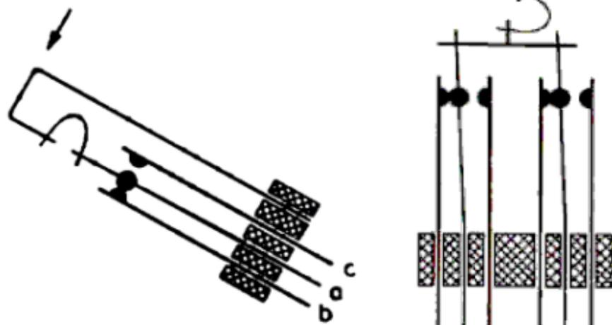
The danger with pushbuttons or switches that are not equipped with spring contacts is that low contact pressure and an insufficiently wide contact gap can cause increased wear and lead to "burn-out". The chance of "burn-out" increases if the switch without spring contacts is not operated manually, but slowly by means of a cam or lever, which is particularly the case with slow-running machines. The "micro-switch" has therefore been designed for these types of applications.
