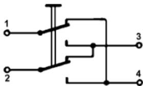
Circuit Diagram of polarity switch
