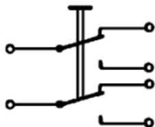
Such a "2-pole" change-over switch is often used as a "pole reversing switch" for reversing the direction of rotation of DC motors. The fischertechnik switch has already been wired in this configuration at the factory.
