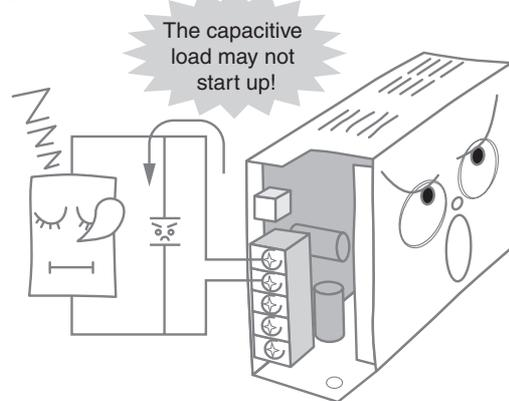
\* For details, refer to *An output delay occurs in the output turning ON* in the Problem column of the table on page 18.
