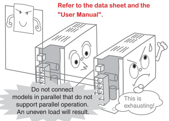
\* For details, refer to *Series, parallel, and ± output operation* in the *Check point* column of the table on page 15.
