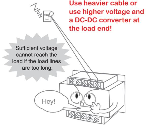
\* For details, refer to *The voltage applied to the load is low.* in the *Problem* column of the table on page 19.
