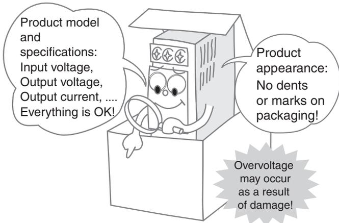
**Always bench test a power supply and check that it can provide the voltage and current required plus check it has the features required. e.g. overload operation, voltage adjustment range etc. For further information see the "User Manual".**
