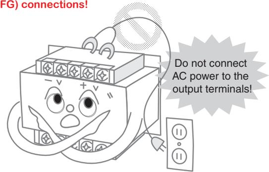
\* For details, refer to *Input terminals* in the *Check point* column of the table on page 15. Use an RCD device during testing!
