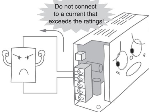
**Disconnect the load and try the power supply again.**
