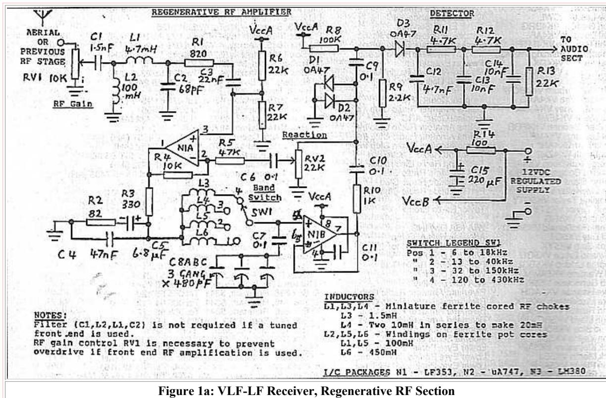
Figure 1a: VLF-LF Receiver, Regenerative RF Section
