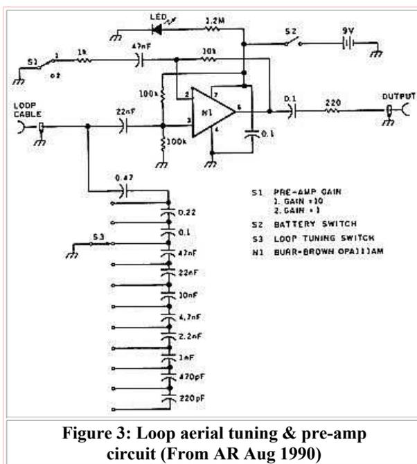
Figure 3: Loop aerial tuning & pre-amp circuit (From AR Aug 1990)
