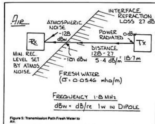
Figure 5: Transmission Path - Fresh Water to Air.
