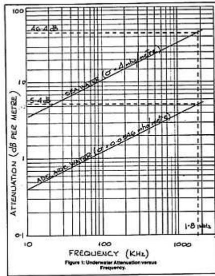
Figure 1: Underwater Attenuation versus Frequency.
