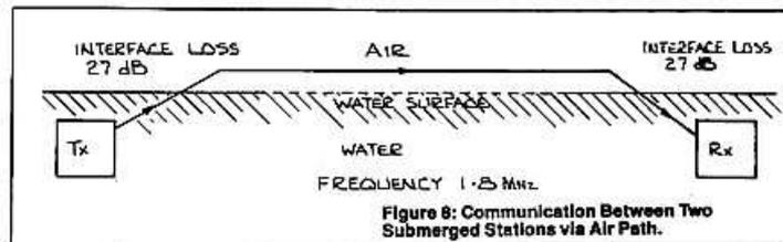
**Figure 8. Communication Between Two Submerged Stations via Air Path.**
