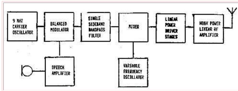
**Fig 6 - Typical single sideband transmitter.**
