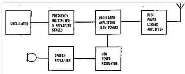
**Fig 5 Low Level Amplitude Modulation Transmitter.**
