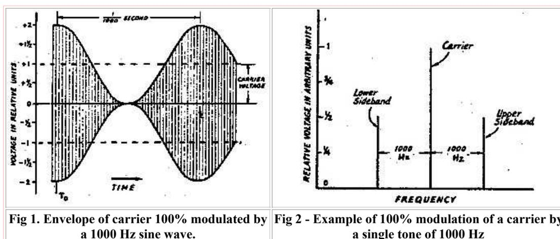
Since power is proportional to the square of voltage, the proportion of power in each side frequency is equal to 0.5 squared or a quarter of that in the carrier. If the carrier is modulated 100 per cent by a complex waveform of many frequencies, two sidebands of
