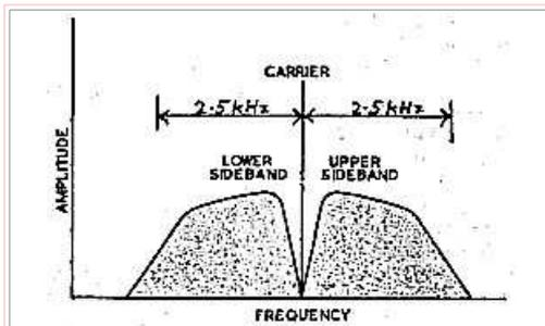
Fig 3 - Amplitude/frequency relationships of carrier and sidebands with 100% speech modulation.
