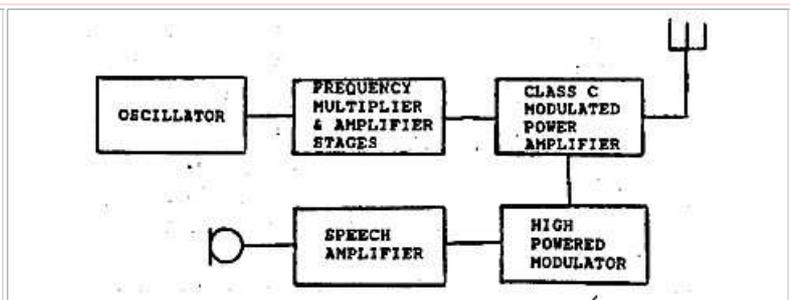
Fig 4 - High level (plate modulated) amplitude modulation transmitter.
