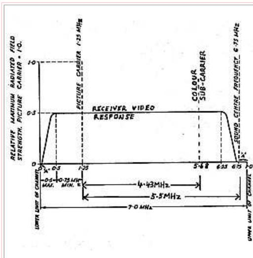
Fig 10 - PAL television signal format.
