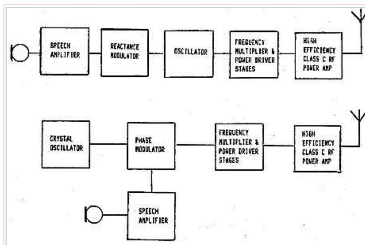
**Fig 9 - Typical frequency modulation transmitters.**
