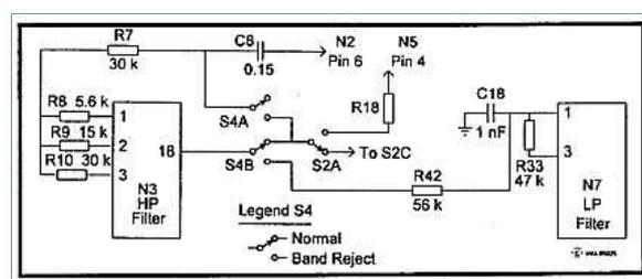
Figure 4 - Changes to the original circuit to include the Band Reject function.
