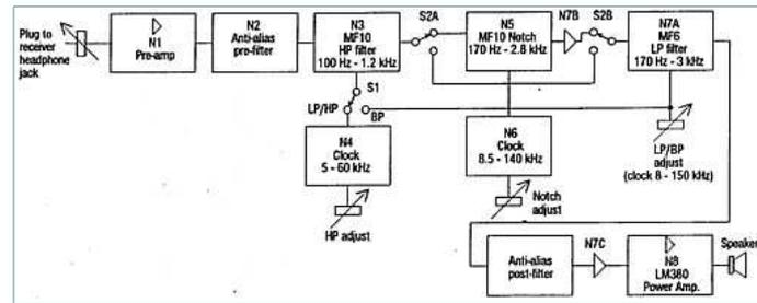
Figure 2 - Audio filter unit - Block diagram.
