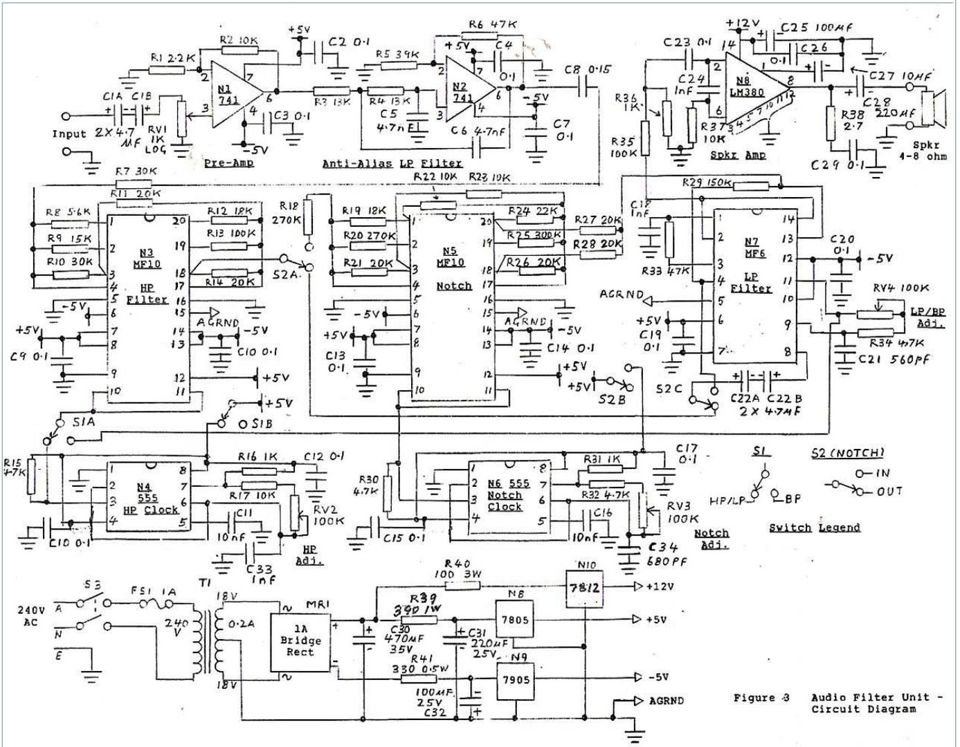
Figure 3 Audio Filter Unit - Circuit Diagram
