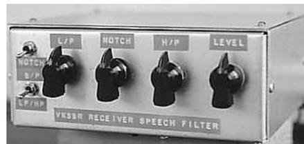
Front panel view of the original receiver filter unit. Not shown are frequency calibration scales added with the modifications, Part 2
