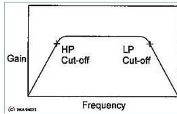
Figure 1 - Normal sequential operation of HP and LP filters with cutoff frequencies set for a wide bandpass.
