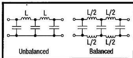
Figure 1 - Typical passive lowpass filters.
