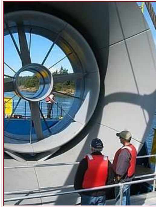
Photo 4 Tidal Current Turbine before installation at Racerocks, British Columbia, Canada (From EnergyBC Ref. 6)
