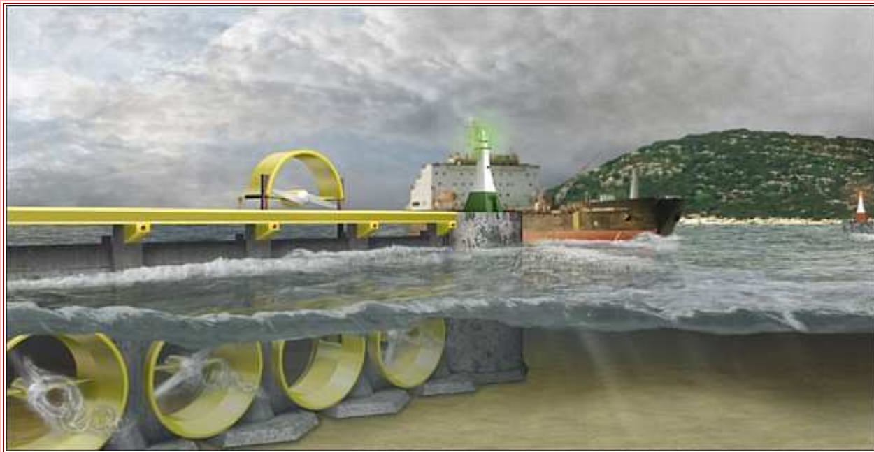
Figure 7 - Energy from tidal currents Artist's rendition of a tidal fence (From EnergyBC Ref. 6)
