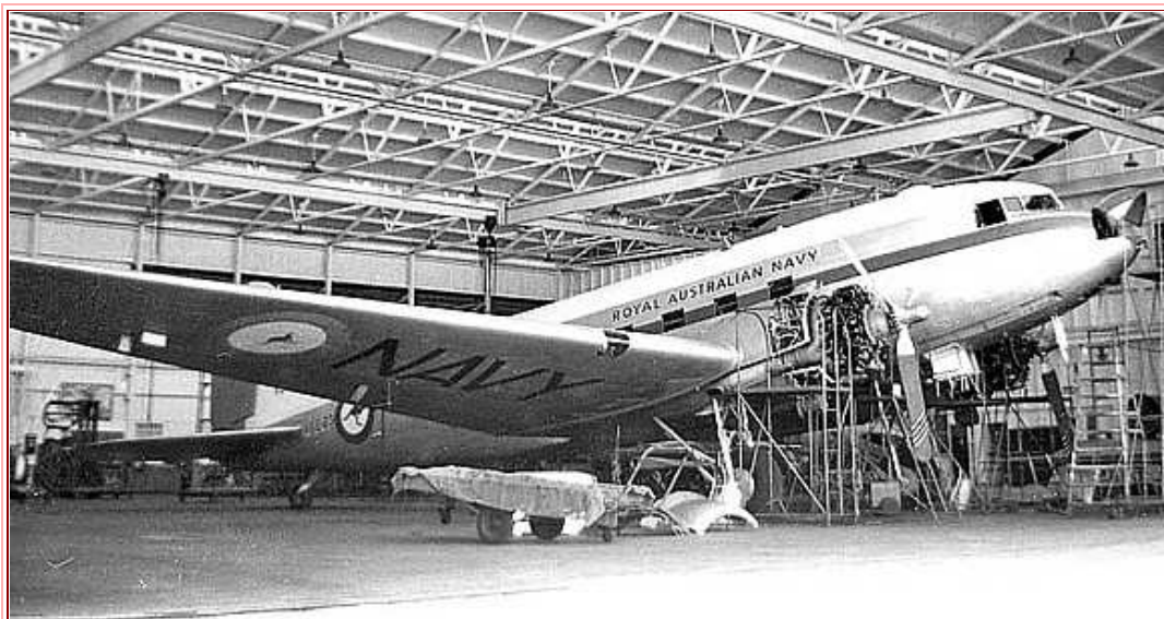
Photo 19 - C47 (DC3) aircraft refit in the DAP hangars 1961 (Goodall Photos - Ref. 8)
