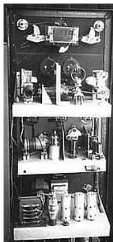
Figure 10 Modulator and RF units at VK5BR.
