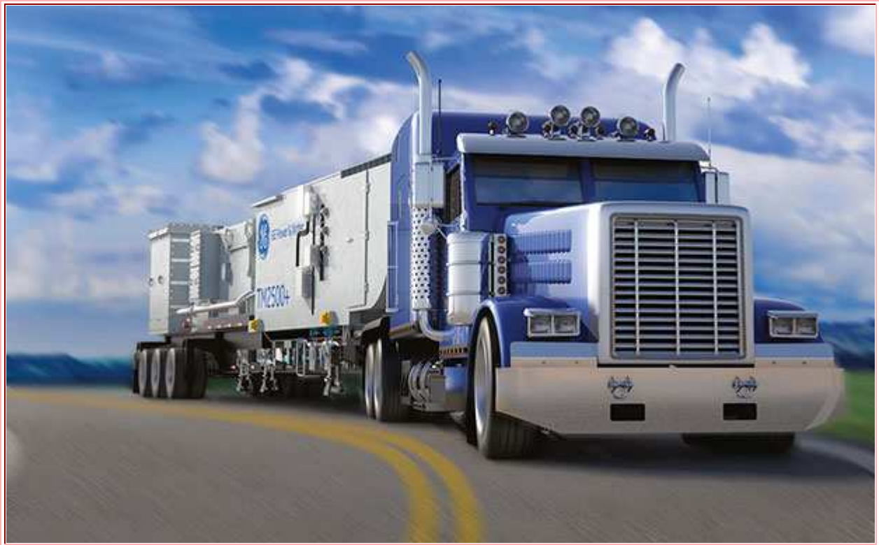
General Electric TM2500 Generator - can be transported via land.
