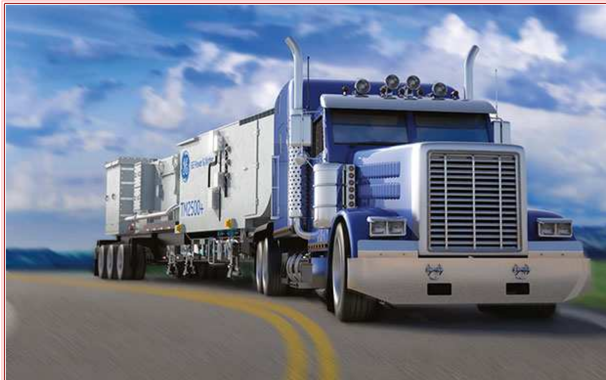
General Electric TM2500 Generator - can be transported via land.
