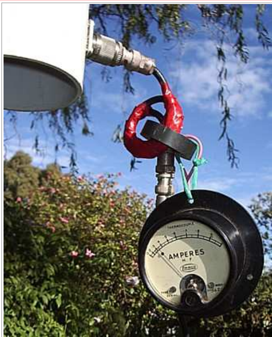
Photo 1 Measuring of Common Mode Current on the Coax at the input to an EH Antenna
