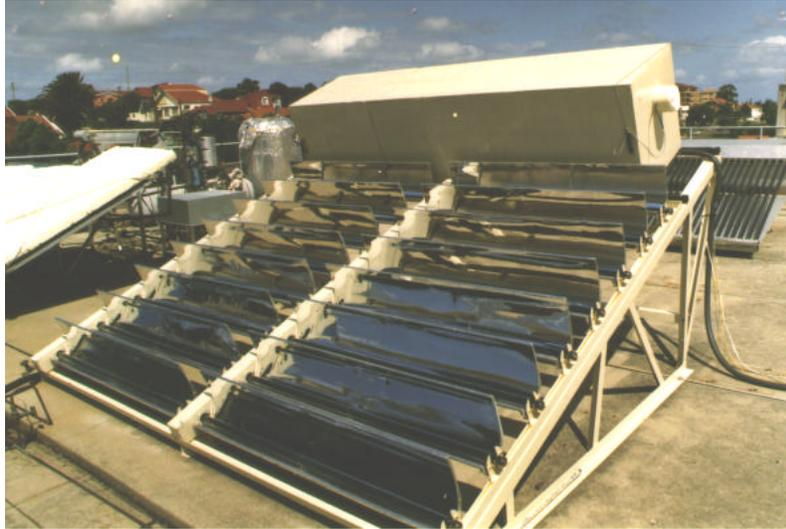
Prototype solar water incorporating stationary mirrors to give winter biased peak performance.
