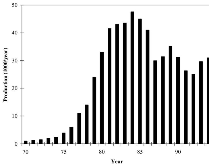
Fig 1. Australian solar water heater production.
