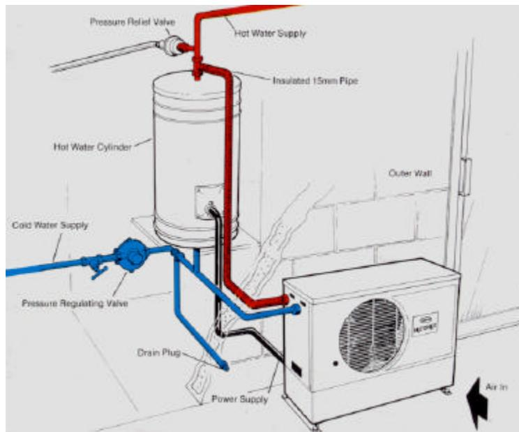
Separate heat-pump air-source water heater.
