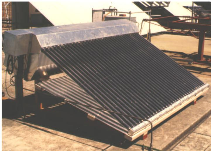
Prototype evacuated tubular collector solar water heater
