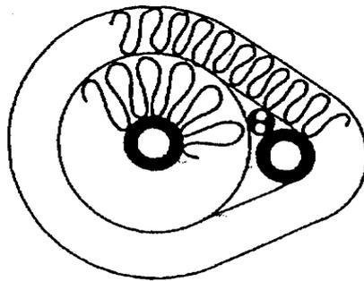
Fig. 1 Cross section of flexible integrated collector-tank interconnection
