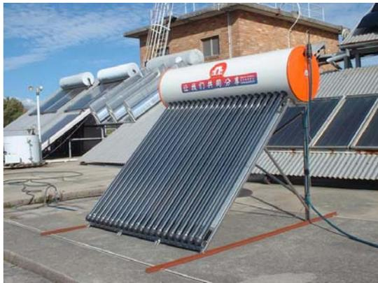
**Figure 1. Water-in-glass evacuated tube solar water heater under test at Solar Thermal Energy Laboratory UNSW**
