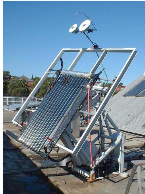
**Figure 4. Experimental setup: Optical efficiency measurement**
