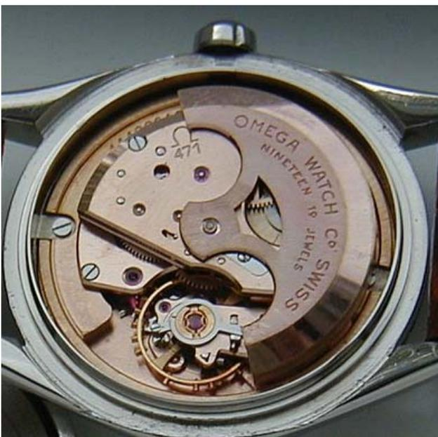
Omega calibre 471 from a Seamaster. Notice the absence of Swan Neck regulator and presence of redundant regulating screws on the balance wheel.
