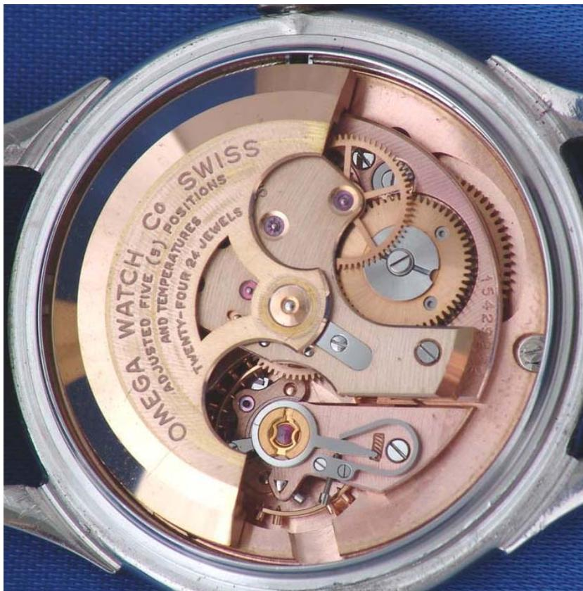
Calibre 505 Movement with redundant regulation screws on the balance. Notice the "Adjusted" script on the rotor. Observe also the earlier version of the swan neck micro-regulator that differs from later 564 series regulators
