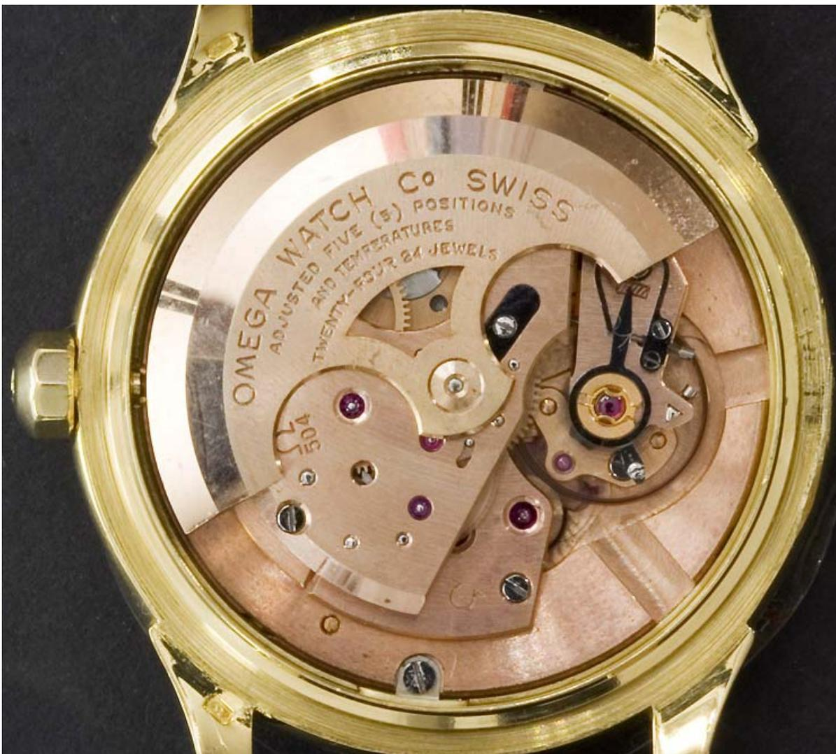
Calibre 504 - date model 24 jewels: Notice the calibre number is stamped on the rotor bridge as opposed to the train bridge
