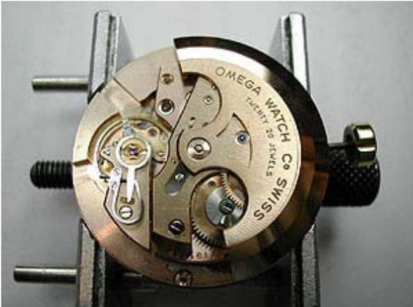
Omega calibre 503. Notice absence of 'Adjusted to five (5) positions and temperatures' that appear on chronometres
