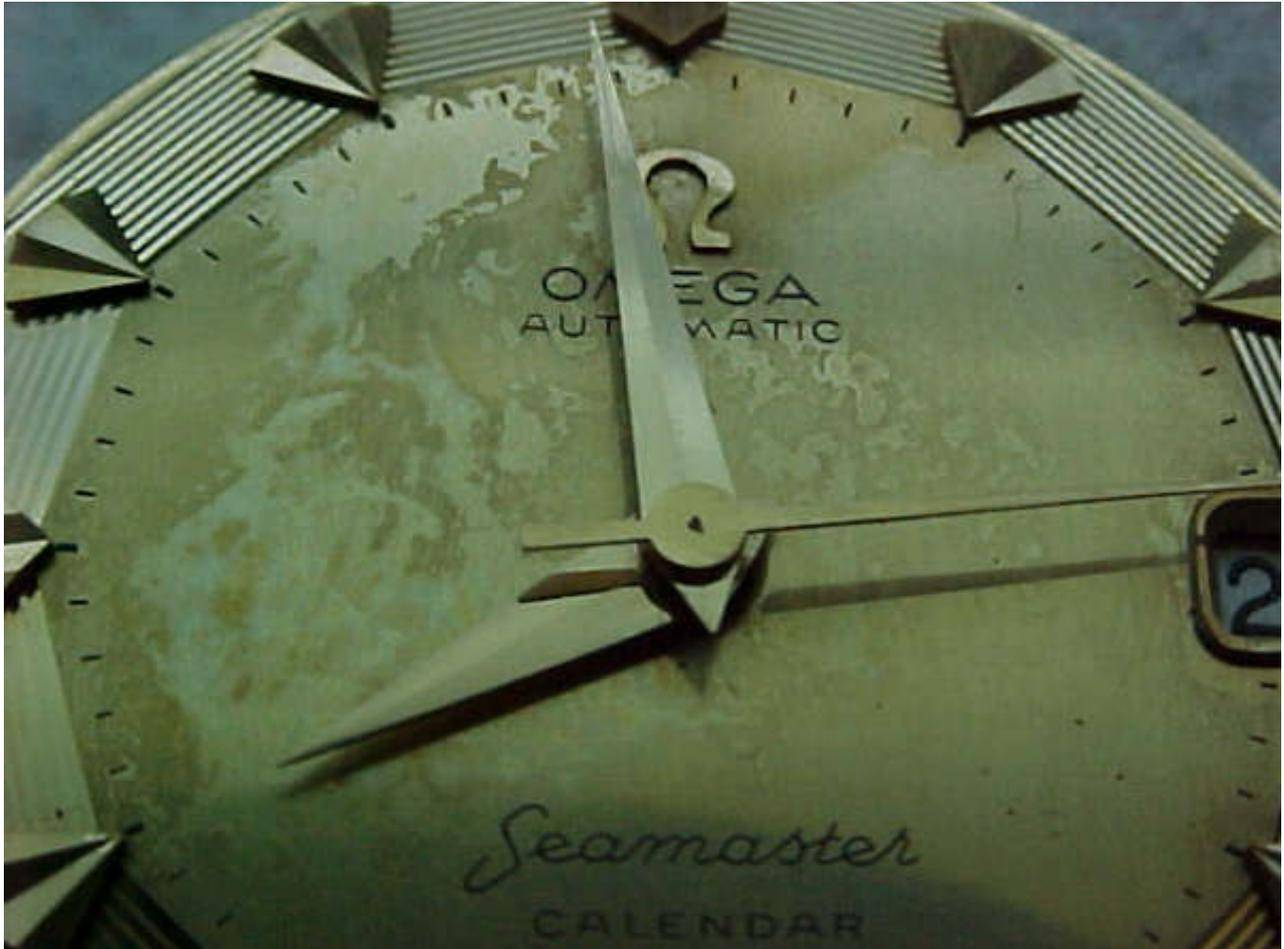
Close-up of dial indicating water damage and some sun-caused degradation of the dial lacquer
