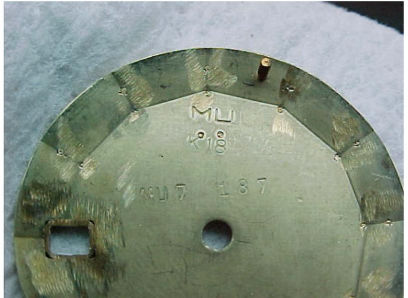
Dial back showing 18K solid gold markings, brushed, hand-applied rivets: proving the dial was original and that the rivets had not been removed prior to a refinishing job.
