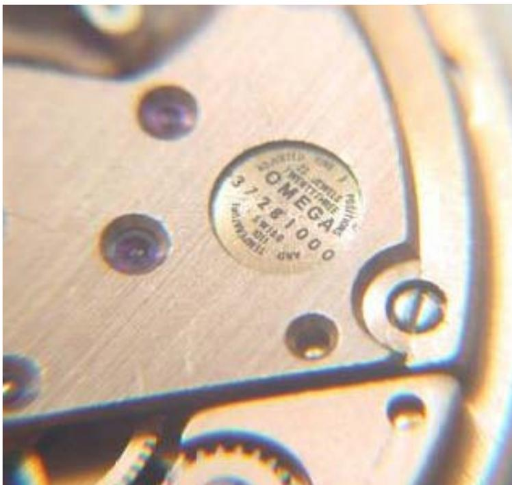
Bridge of a later calibre 1011 showing the decal with serial number, calibre number and adjusted script
