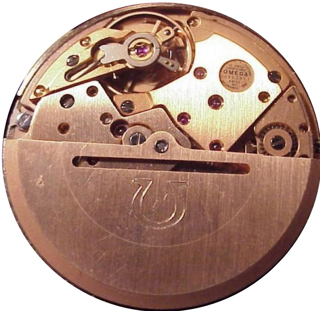
Calibre 1011 Chronometre movement. Notice the simple grained finish of bridges and rotor, inelegant regulator and micro screw, but, nevertheless, the aesthetics of this movement can be pleasing to the eye
