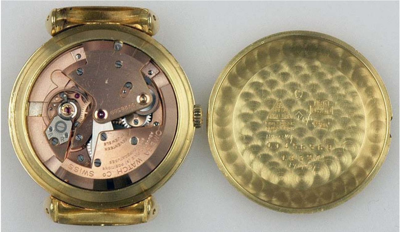
Calibre 352 worked up to chronometer status with rare RG microregulator. DeLuxe Constellation chronometer model OT 14327 Confirmed genuine by Omega
