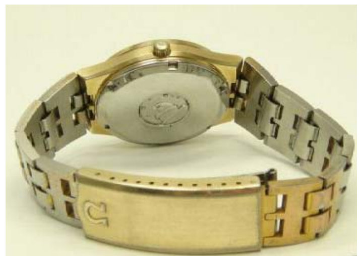
1970s F300 gold electroplated watch head and bracelet. Note the wear in bracelet. The 80 micron watch head is in good shape
