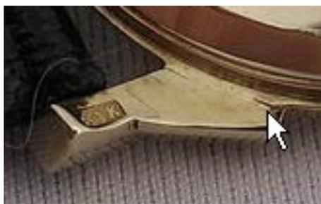
Now let us look at how the movement is fixed to the case. The first picture shows how the filthy, rusted and hopelessly corroded movement is attached by a roughly made case clamp with a burred and rusted screw. Observe the incorrect spacers used on either side of the case clamp. Review the case clamp used on a genuine case and observe how the movement fits snugly into the recess.
