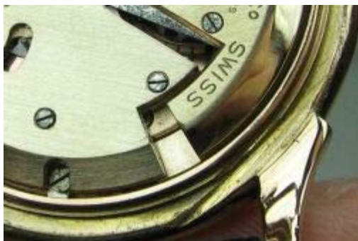
Note groove in case near the lug caused by reckless over-polishing to remove corrosion
