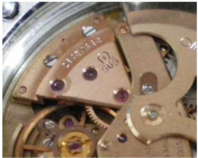
Movement from a franken watch in the wrong 167.005 case. Notice the wheel bridge carries a newer looking calibre 565 bridge. This may have originally been a calibre 564 in need of repair.. Cal 565 never power Omega Constellations
