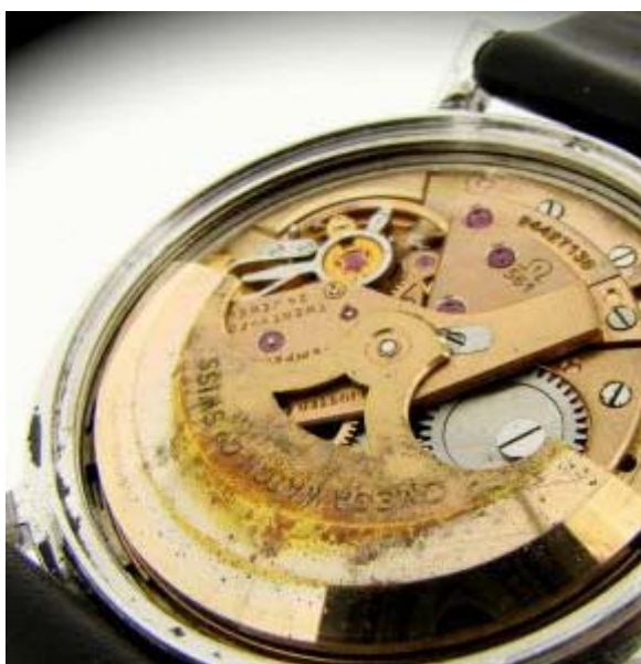
Corroded rotor caused probably by exposure to seawater or other corrosive liquid
