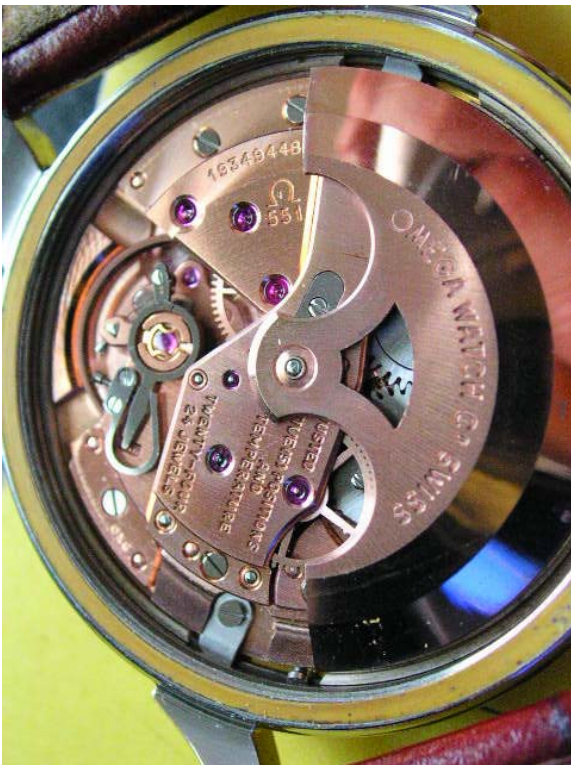
Clean regularly serviced calibre 551 movement. Note all parts are the same colour hue and absence of rust. All correct markings appear.
