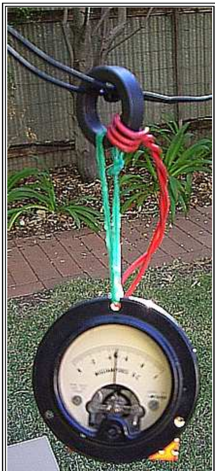
Figure 8 Measuring of Common Mode Current on open wire line to the X3 Antenna
