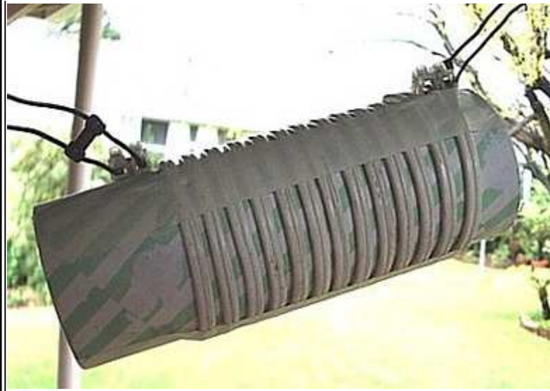
Figure 6 - Balanced Trap for 20 Metres
